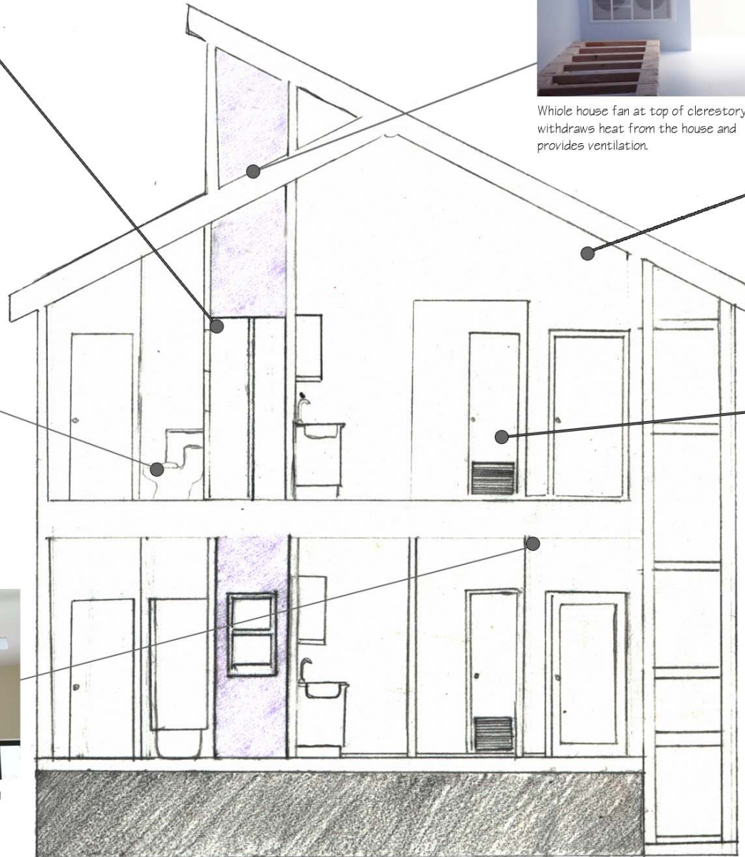
Unfinished shaft section allows students to see the components of the building system.
